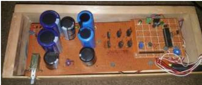
Fig. 5 The Z-source inverter board and Microcontroller board
